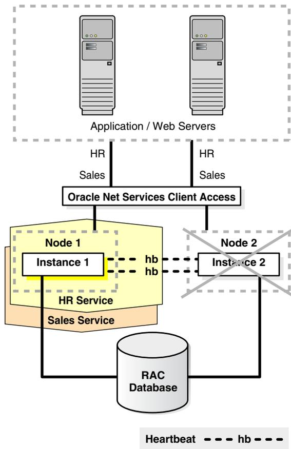
If one Oracle RAC instance fails, then the service and existing client connections can be automatically failed over to another Oracle RAC instance. In this example, the HR and Sales services are both supported by the remaining Oracle RAC instance. In addition, you can route new client connections for the Sales service to the instance now supporting this service.
