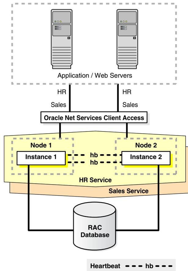
If one Oracle RAC instance fails, then Oracle Clusterware moves the services that were running on the failed instance. If one Oracle RAC instance fails, new client connections are only accepted on the remaining instances that offers that service.
